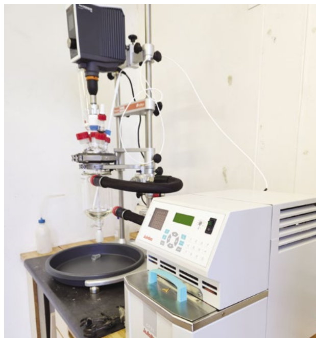
Radleys Single jacketed 1 L Process Reactor for laboratory scale up in a plant-simulated environment. Image: Louise Hamilton
