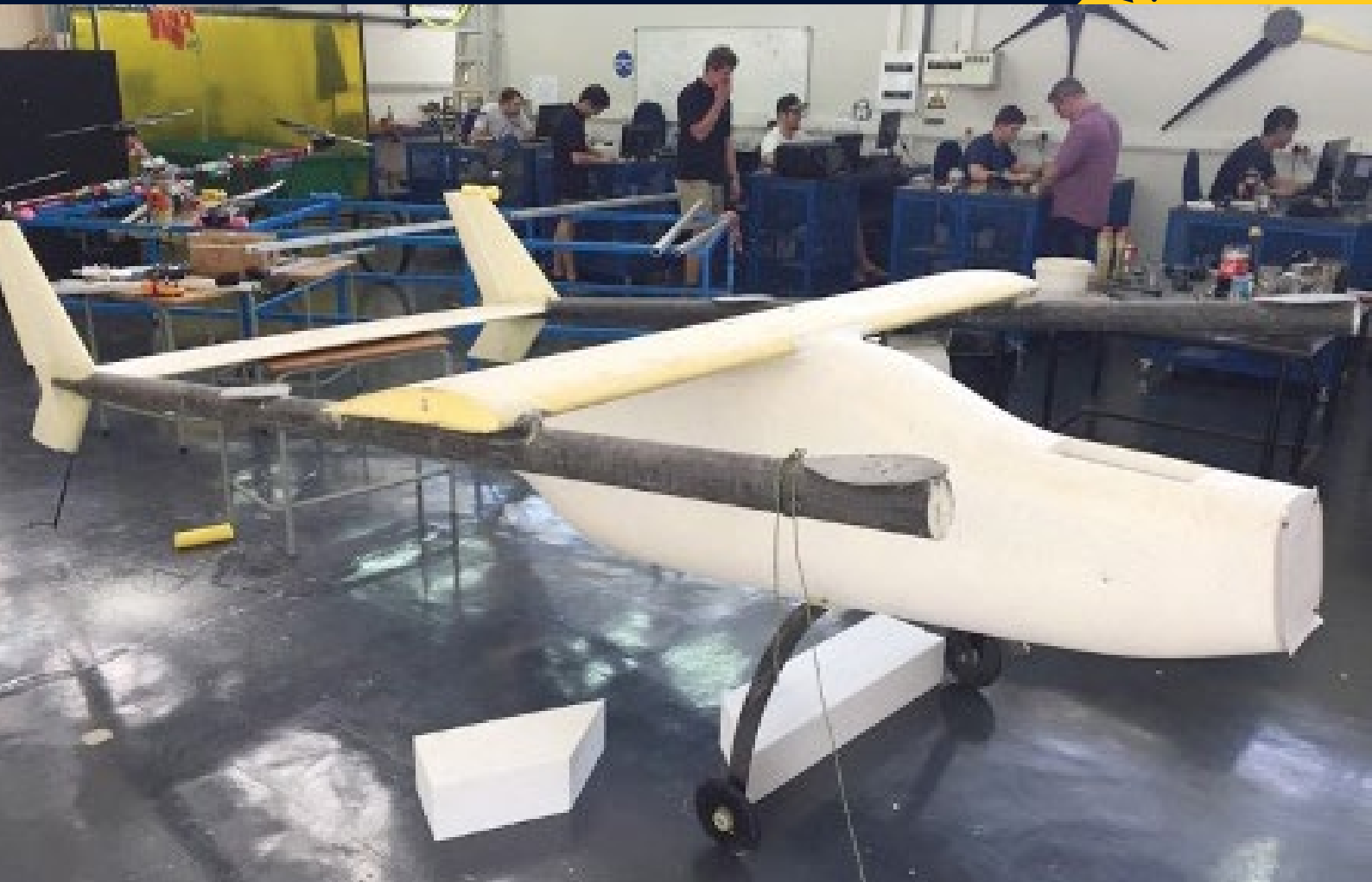
Nelson Mandela University prototype under construction (7,5m wingspan)
